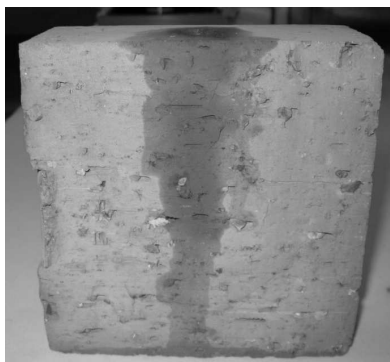
Fig. 1 Ceramic brick filled by siloxane injection
