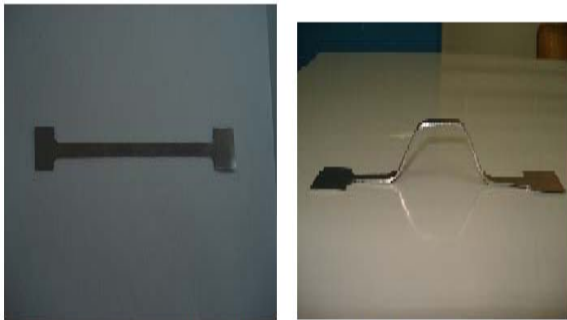
Fig. 3 (a) Form of specimen before and after unloading
