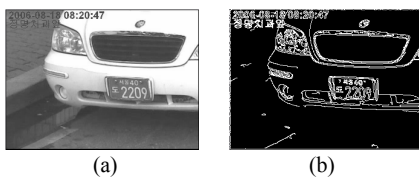
Fig. 2 Preprocessing, (a) Gray image from color input image, (b) Edge image from (a)
