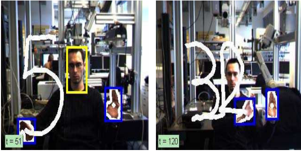
Fig. 6. Gesture path for isolated number 5 and continuous number 32 from connected centroid points of hand regions.
