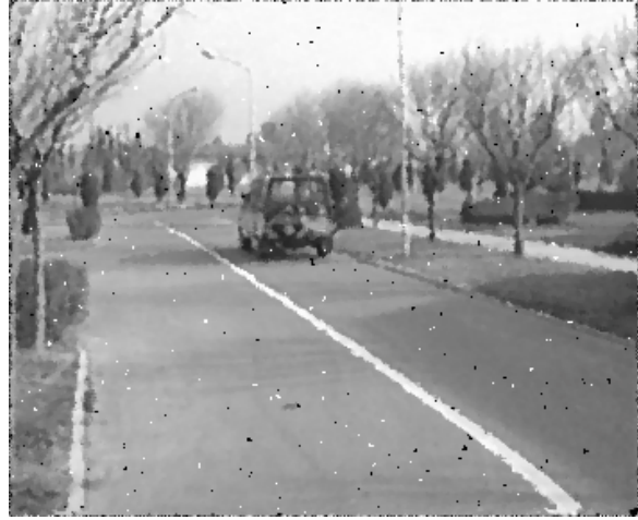
Fig. 3(e). Filtered frame 335 of moving Patrol after applying our proposed fuzzy filter using N=3 frames under 50% noise density
