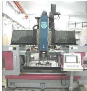
Fig. 3 NC incremental forming machine
