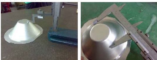
Fig. 6 Diameter measurements along the contour layers
