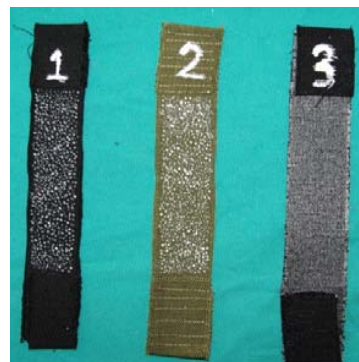
Fig. 1 Example Specimens prepared for uniaxial tensile testing
