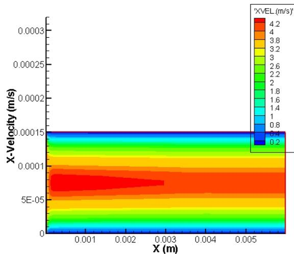
Fig. 4 Contours of the axial velocity component
