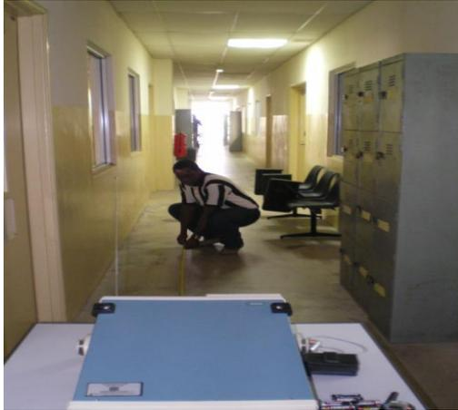
Fig. 11: Emmanuel Ojakominor takes measurements in environment I. Notice the make-up of the environment, having a number of (glass) windows at both walls, as well as objects such as metallic lockers located at adjacent positions along the passageway.
