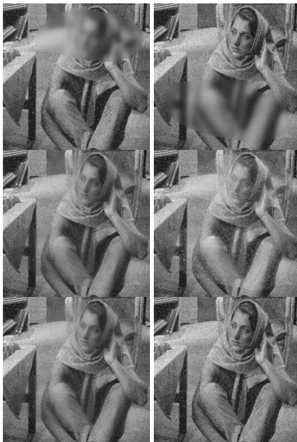
Fig. 3. Fusion results, the original image randomly blurred, with Salt and Pepper noise added. Top row: input image X (left), input image Y (right). Second row: fused image F using averaging (left), fused image F using ratio pyramid decomposition (right). Bottom row: fused image F using the PCA decomposition (left), fused image F using DWT domain fusion (right)
