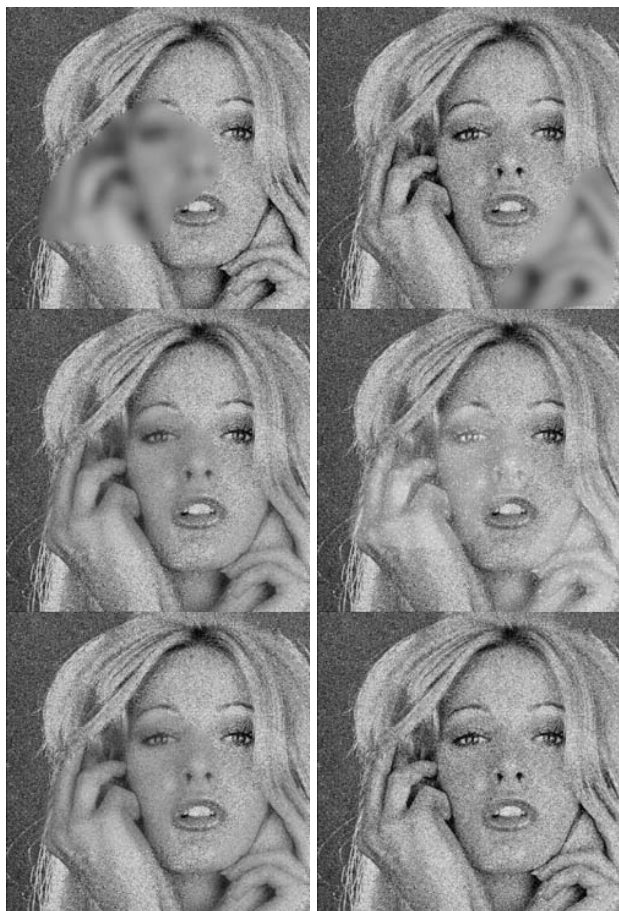
Fig. 2. Fusion results, the original image randomly blurred, with Gaussian noise added. Top row: input image X (left), input image Y (right). Second row: fused image F using averaging (left), fused image F using ratio pyramid decomposition (right). Bottom row: fused image F using the PCA decomposition (left), fused image F using DWT domain fusion (right)
