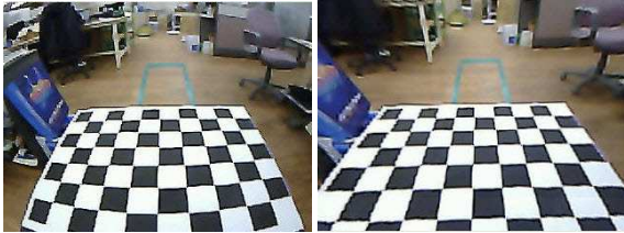
Fig. 3 Image-Plane with lens distortion correction Left- raw image plane, Right- lens distortion correction image
