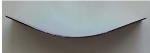
Fig. 7 Silicon foil shaped with a pressing mold of radius 75 mm
