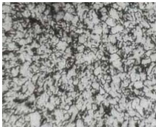
Fig. 1 Optical micrographs (a) base metal (b) heat affected zone and (c) weld metal deposited at a current value of 150A
