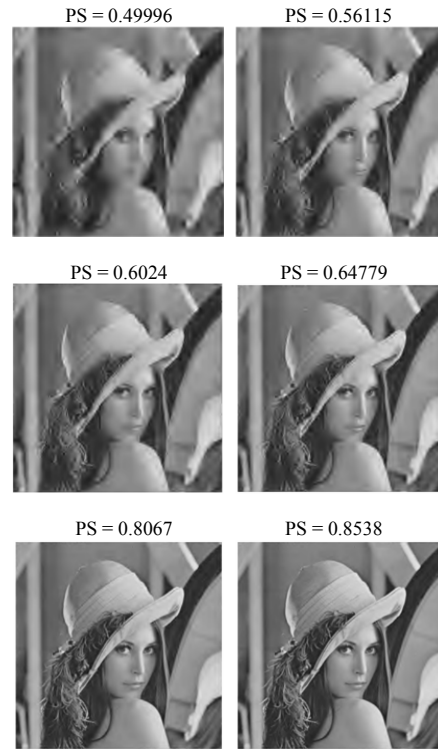
Fig. 9 “Lena” image compression results. The images of the left column that follow are for SPIHT ONLY coded images. The images of the right column that follow are for the visually optimized SPIHT POEZIC coded images. The bit rates from top to bottom are 0.0625 bpp, 0.125 bpp and 0.5 bpp respectively
