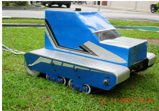
Fig. 6. Developed prototype of air-cushion track vehicle [9]
