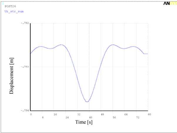
Fig. 33 Vertical displacement  $U_z$ , mid span, Variant No. 10
