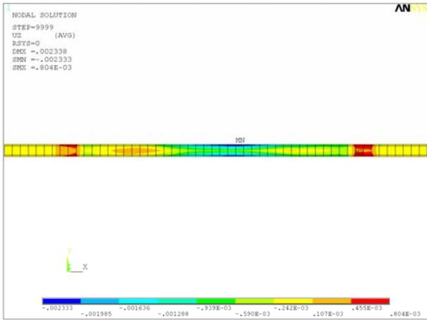
Fig. 28 Maximal envelope  $U_z$  dynamic, Variant No. 3 – torsional
