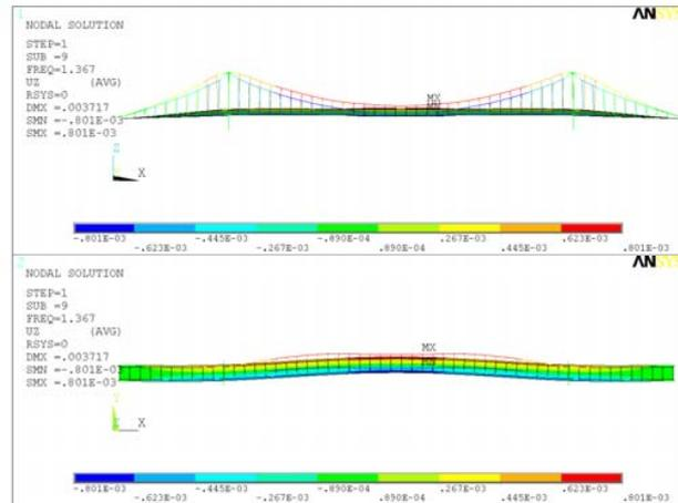
Fig. 12 Eigen shape according to  $f = 1.367 \text{ Hz}$
