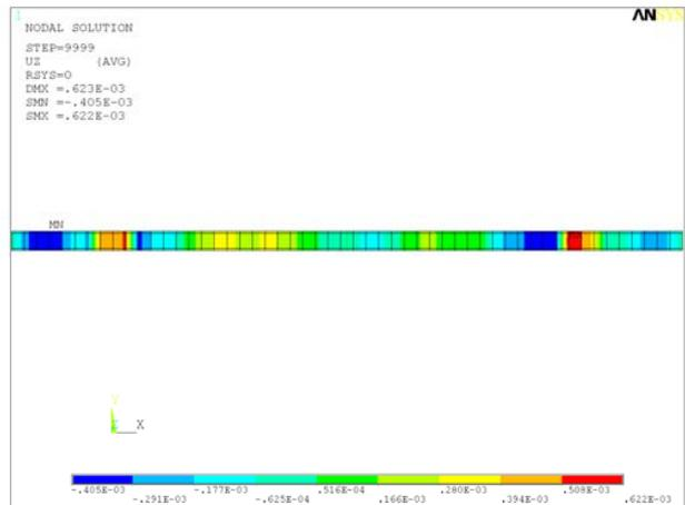
Fig. 26 Maximal envelope  $U_z$  dynamic, Variant No. 9
