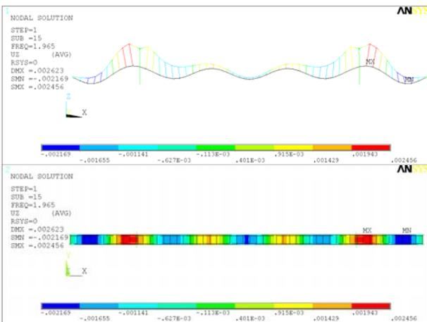
Fig. 15 Eigen shape according to  $f = 1.965$  Hz
