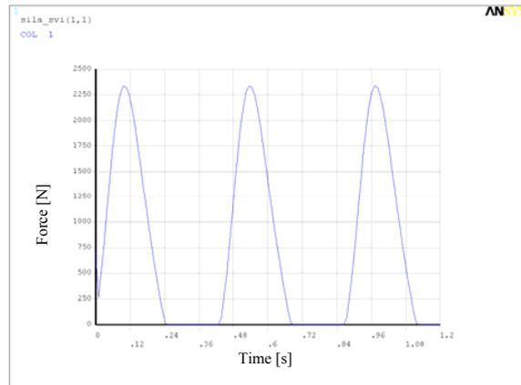
Fig. 21 Vertical force time record for running
