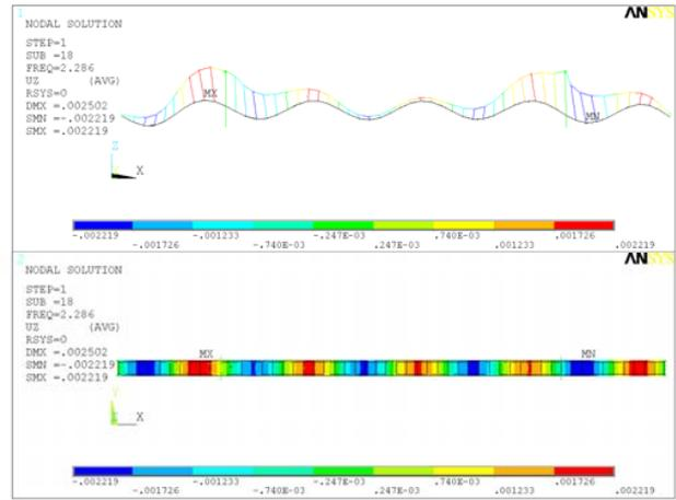
Fig. 17 Eigen shape according to  $f = 2.286$  Hz
