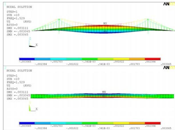
Fig. 13 Eigen shape according to  $f = 1.529 \text{ Hz}$
