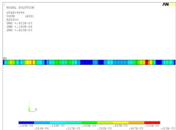
Fig. 27 Maximal envelope  $U_{SUM}$ , Variant No. 9
