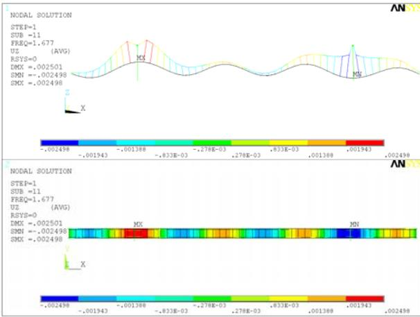
Fig. 14 Eigen shape according to  $f = 1.677$  Hz
