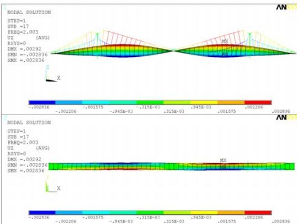
Fig. 16 Eigen shape according to  $f = 2.003$  Hz
