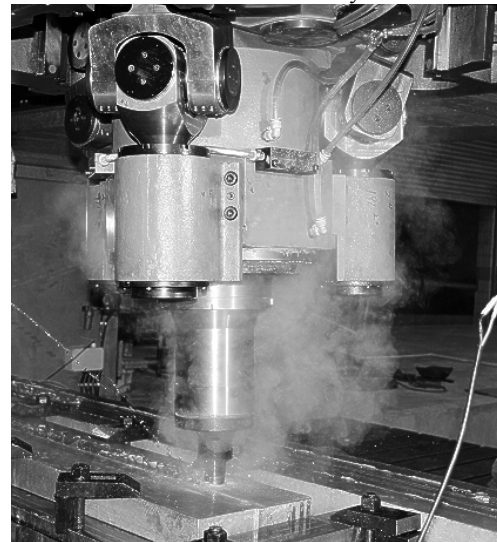
Fig. 9 Prototype of the proposed tool head for friction stir welding
