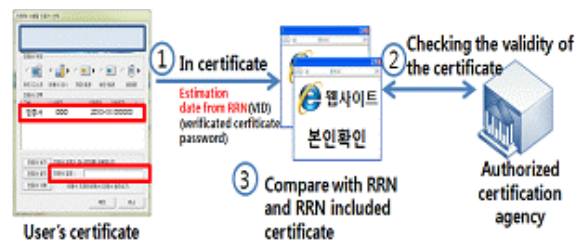
Fig. 1 Certificate authentication using RRN
