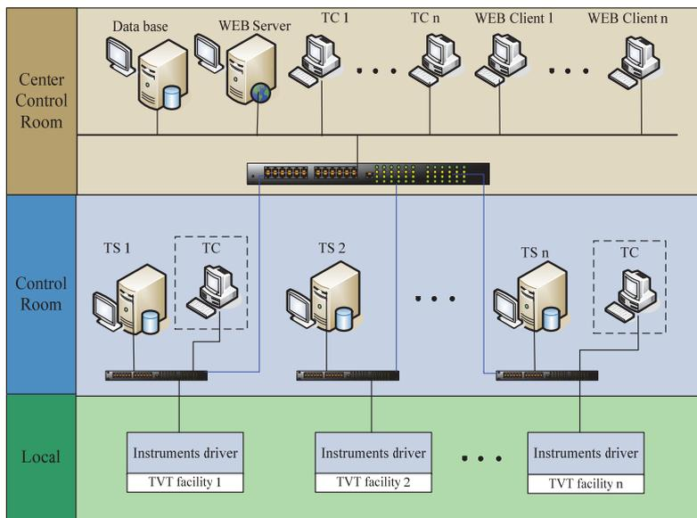
Fig. 5 Centralized mode
