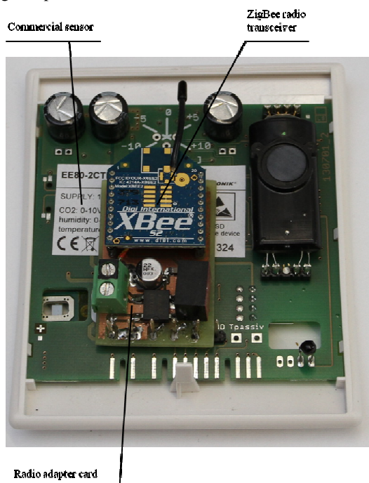
Fig. 2 Commercial sensor (E+E Elektronik, EE80) has been modified to wireless using radio adapter card and ZigBee radio transceiver (Digi International Inc., XBee PRO S2B)
