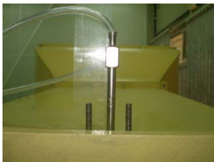
Fig. 9 Height adjustment of the Pitot tube
