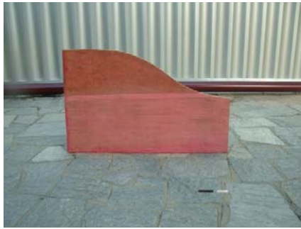
Fig. 1 Molds for the diffuser
