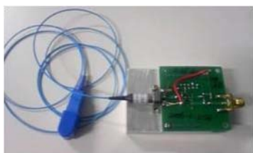
Fig.2 Configuration of ROSA PIN-PD with Pre-Amplifier
