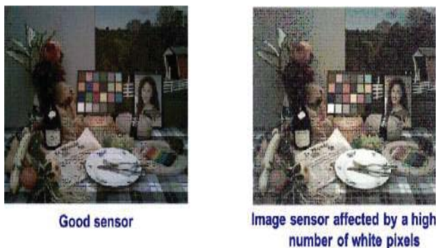
Fig. 1 Metallic ions contamination in DTI leading to the apparition of white pixels
