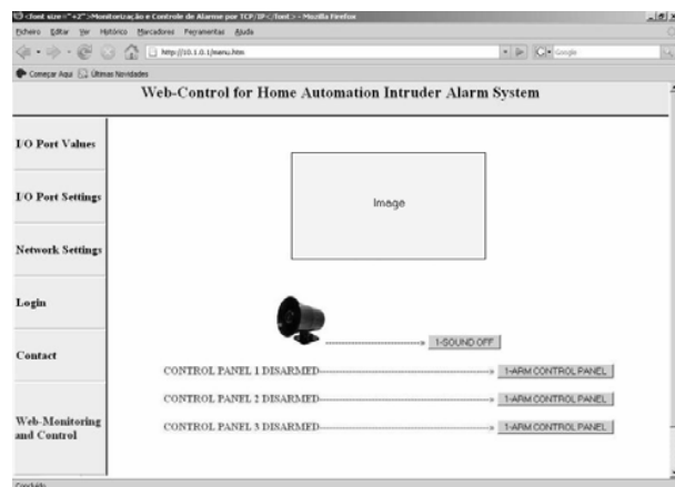
Fig. 9 Web-control for a home automation alarm system
