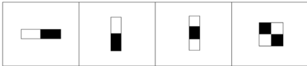
Fig. 7 Feature prototypes of simple Haar-like. Black areas have negative and white areas positive weights .
