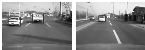
Fig. 10 Same directional vehicle detection of using haar-like and adaboost.
