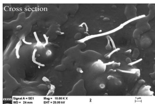
Fig. 7 SEM image of composite cross section
