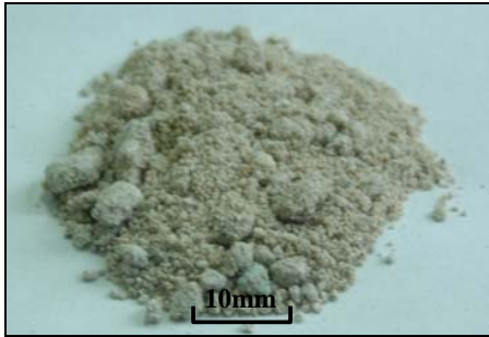
Fig. 1 Image of the reducing slag before grinding
