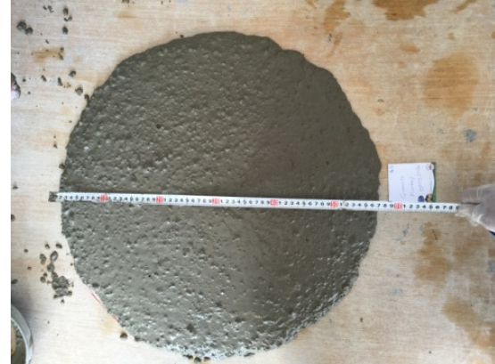
Fig. 3 Flow and T 50 time testing
