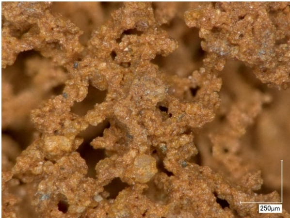
Fig. 2 CCF structure micrograph, optical microscopy, at X200 magnification
