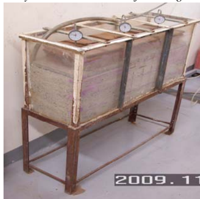
Fig. 1 Model shape with volume change measuring unites
