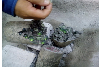
Fig. 5 Internal bond in Concrete cylinder
