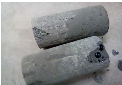
Fig. 4 Crack pattern in Concrete cylinder
