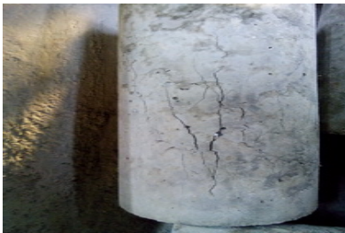
Fig. 3 Crack pattern in Concrete cylinder
