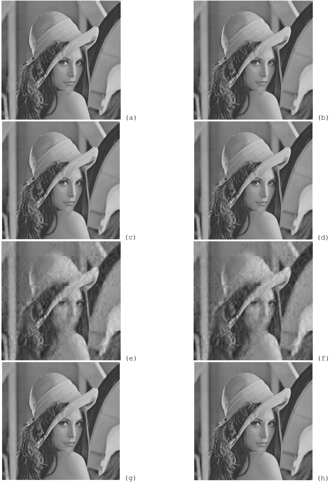
Fig. 14 Comparison of compression techniques: (a) original, (b) Haar, (c) Haar + Morton's scan, (d) Haar + row-rafter scan, (e) Morton's scan + KLT, (f) row-rafter scan + KLT, (g) Haar + Morton's scan + KLT, and (h) Haar + row-rafter scan + KLT
