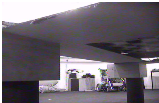
Fig. 7 Test mobile robot vision at under vehicle inspection (Dimension 4*2 meters)
