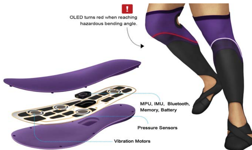
Fig. 4 Hands-free feedback delivers to insoles and kneepad by vibrations and lightening
