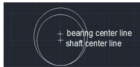
Fig. 1 Bearing center line and shaft center line position in shaft sleep condition
