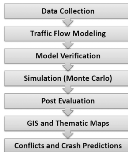
Fig. 2 Process Flow diagram for Crash Prediction
