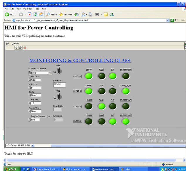
Fig. 5 Controlling the system remotely
