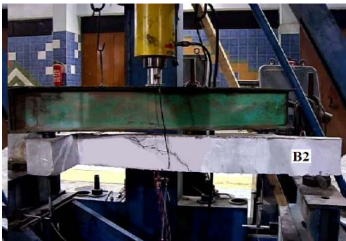
Fig. 4 (c) Failure modes and crack patterns of the tested beam B2
