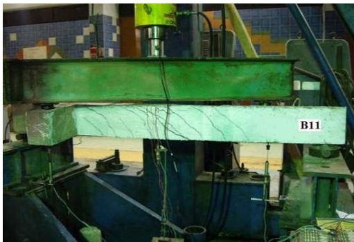
Fig. 4 (a) Failure modes and crack patterns of the tested beam B11
