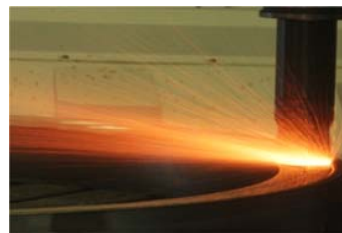
Fig. 1 High speed milling process using ceramic cutting tools
