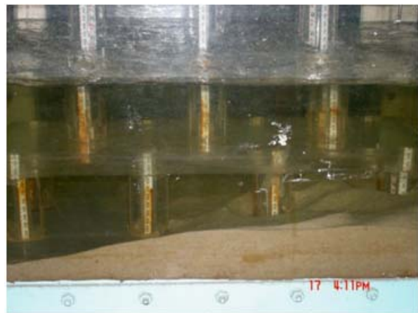
Fig. 12 Maximum scour depths at piers and combined piles after 24 hour
