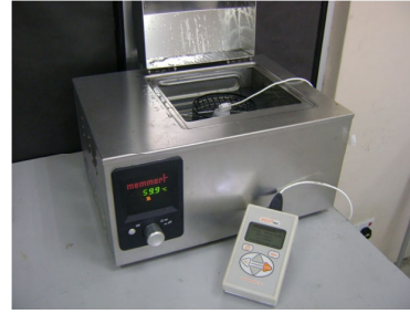
Fig. 1 Thermal conductivity measurement using KD2 Pro Thermal Analyzer
