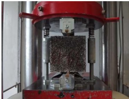
Fig. 3 Splitting tensile test
