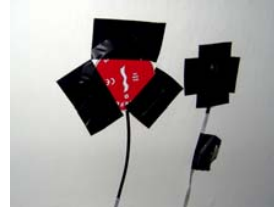
Fig. 5 Heat flux sensor and contact temperature probe
