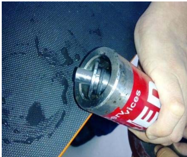
Fig. 3 Leakage inside the connector
