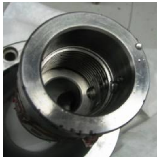
Fig. 7 Water droplets leaked deep in interconnect
