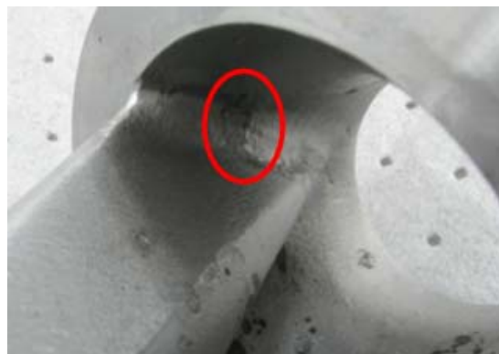
Fig. 4 Suspected casting defect area
