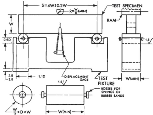
Fig. 2 SE(B) Sample and bend specimen [2]
