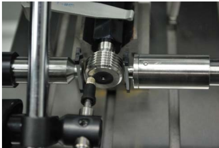
Fig. 7 The pitch diameter of the pipe taper thread measuring with the three-wire probe
