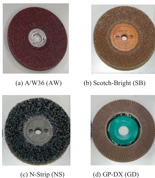
Fig. 2 Polishing agent for surface finishing
