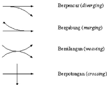
Fig. 1 Image of Transfer of Vehicle Motion [9]
