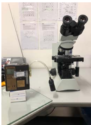
Fig. 13 The air monitoring pump and a filter attached
