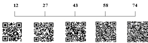
Fig. 4 The quantity of the input characters, respectively in 12,27,43,58 and 72, and their corresponding patterns
